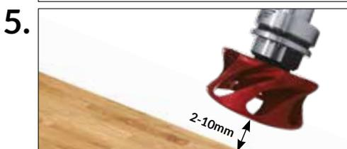
**The usage of a pre-setter device is recommended** to ensure a 2-10 mm gap between the IMS Twister and the work space. If the Twister shows any signs of overheating, make sure to increase the gap between the nut and work space as it may be too close to the cutting surface.
